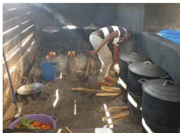
Energy saving OLI-60b cookers have taken over from the old fire-places.
