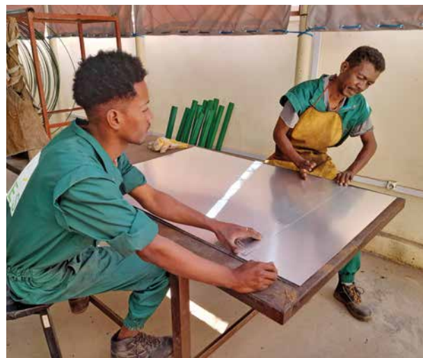
Employees cutting sheet metal in Toliara for parabolic cookers.
