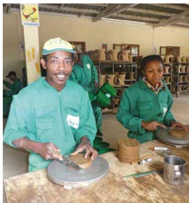
Employees model the clay grates for the energy-saving cookers
